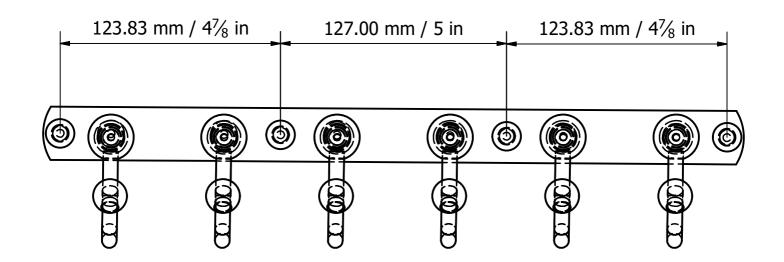
Step2: Attach unit to Mounting Surface.
